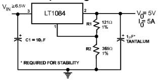
$$V_{out} = V_{REF} (1 + \frac{R_2}{R_1}) + I_{ADJ} R_2$$
